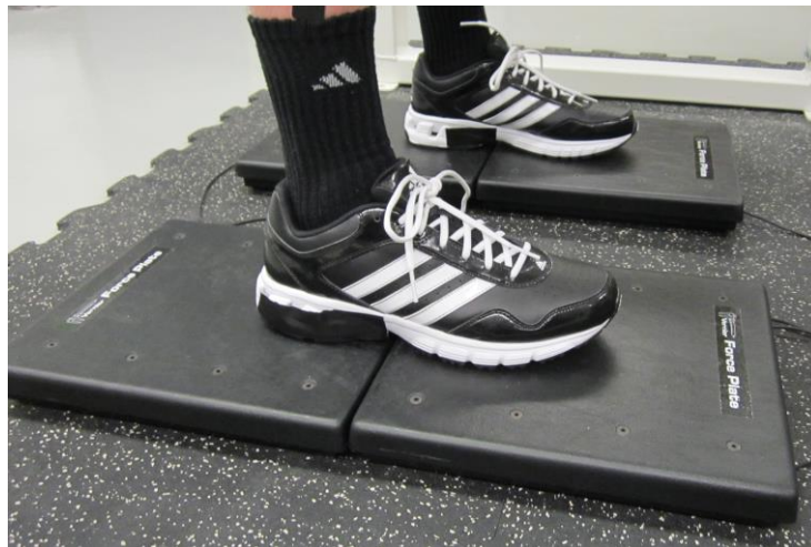
Figure 2. Foot placement for the back squat. Tape marks indicated the location of peak arch height, which was centered over the seam between two plates; thus, force distribution would be in either direction from the seam.
