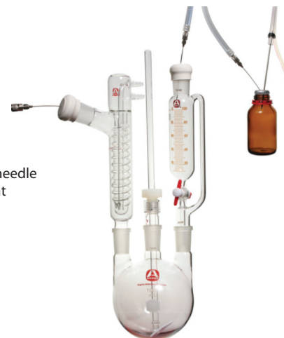
Fig. 13 Double-ended needle transfer with syringe valve
