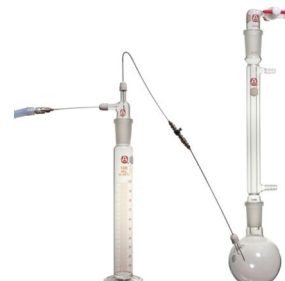
Fig. 13 Double-ended needle transfer with syringe valve
