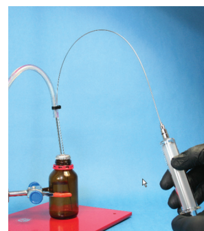
Fig. 8 Filling syringe using nitrogen pressure
